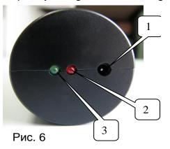
Charging time of a fully discharged battery does not exceed 5 hours (typical value is 3.5 h). In case of a failure (charging is not complete within five hours) a charger switches off automatically, both LEDs will go out.
